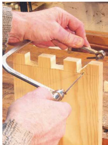
▲ Pic.10 Cutting out waste with a coping saw, but you could use a piercing or fretsaw
